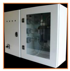
The FTA continually samples the process liquid and creates foam inside a small test chamber which is then measured. The selfcontained unit includes sampling pumps and an anti-foam pump to control the foam. If required the anti-foam pump can be replaced by an intelligent interface to an external process controller.
